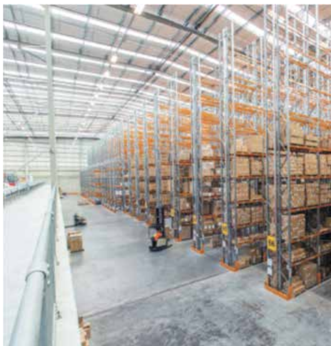
Fig. 3—James Pascoe Group introduced cutting-edge logistics technology to create a state-of-the-art facility. A key feature was the 52 ft (16 m) high VNA racking – the highest ever installed in New Zealand.
