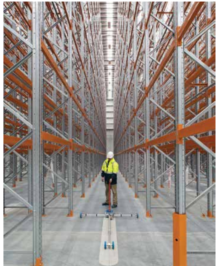
Fig. 5—FACE Consultants Profileograph surveying of the JPL Distribution Center.
