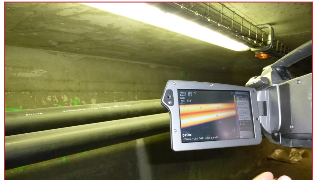
After injection – control with thermal camera (this application was for this jobsite only)
