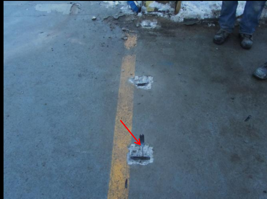
Screw drive penetration test indicating a de-tensioned PT tendon on the flat portion of the Roof Level
