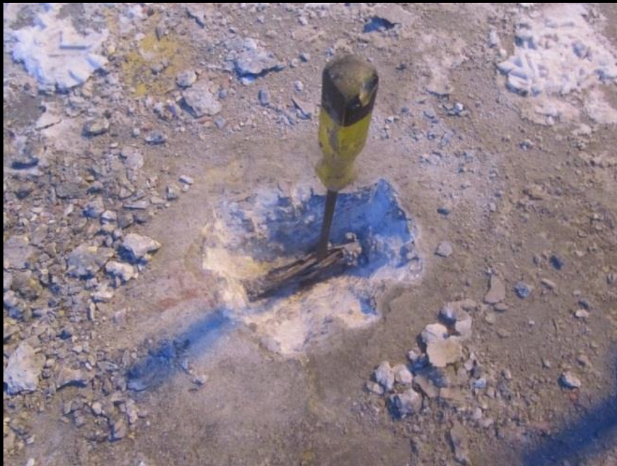
Screw drive penetration test indicating a de-tensioned PT tendon on the ramp at the Roof Level
