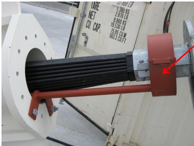
Measuring device bolted to anchorage at deck level
