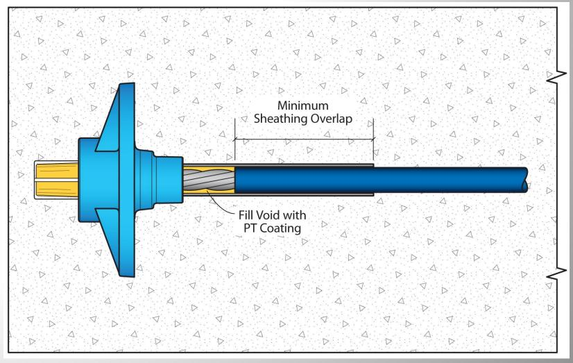
ACI 423.7-14, 6.5.2c) – Within the connecting component or enclosure, either the prestressing steel shall be covered by sheathing for its full length, or the annular space between the sleeve and the strand shall be filled with PT coating.
