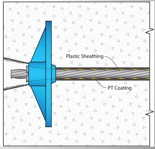
Recently, stressing pocket patches have come to the forefront of challenges in unbonded post-tensioning. This was identified as one of the reasons for the recent demolition of McGuire Apartments in Seattle. The Nadine Post article in ENR states that "McGuire's problems center around corrosion of steel tendons at stressing-end anchors due to a lack of corrosion-resistant paint and non-shrink grout".
