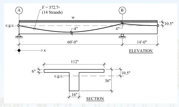
Unfactored Service Loads "w": f'c = 4000 psi Parabolic Tendon Profile
