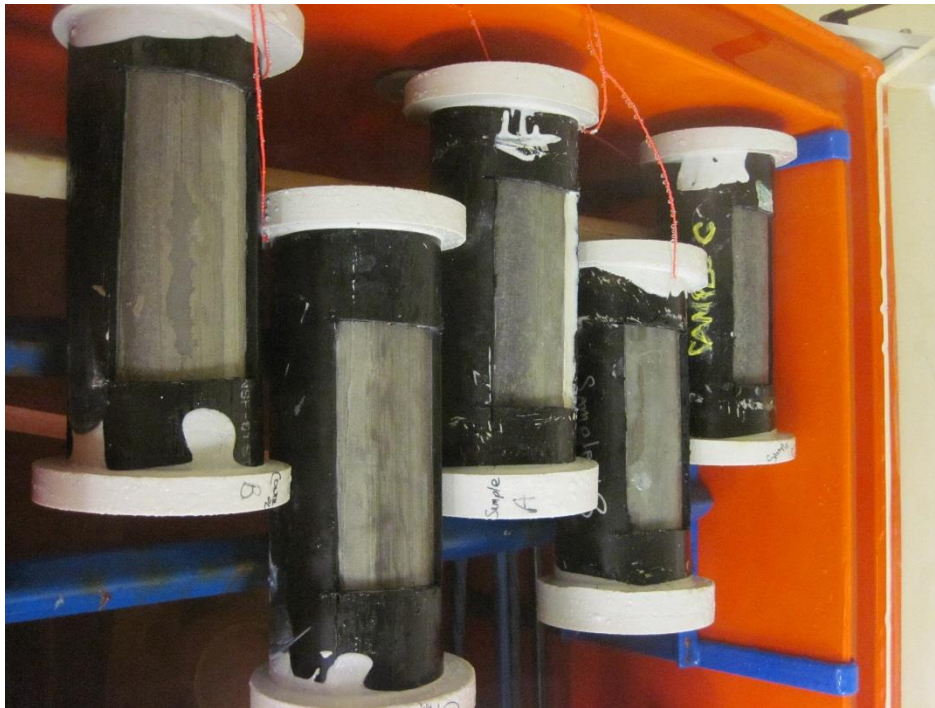
Figure 1: Three impregnated and three control specimens were placed in a salt-fog chamber on mid February 2015. Voltage potentials (CSE) are obtained twice a week to identify time of corrosion initiation.
