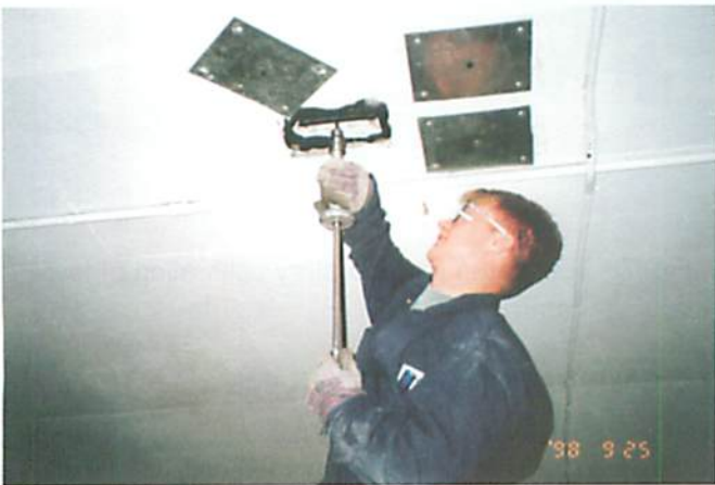
Fig. 2 - Wire penetration (screwdriver) test
