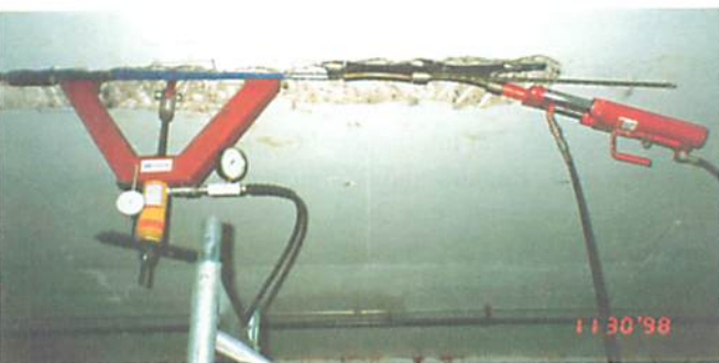
Fig. 9 - Field calibration of the test frame
