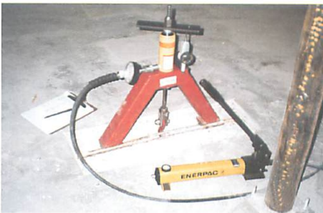
Fig. 6 - In-situ tension test set-up in field
