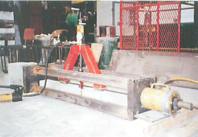
Fig. 7 - Test setup for laboratory calibration of test frame
