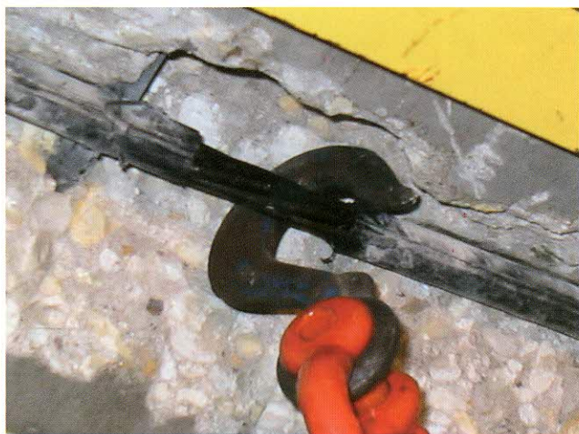
Fig. 6 – Close Up of Test Hook on Exposed Tendon
