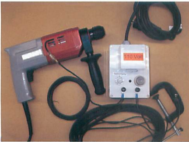
Fig. 2 – Special Drill with Automatic Shut-off Capabilities When in Contact with Metal; Dial Graduates Sensitivity of Instrument
