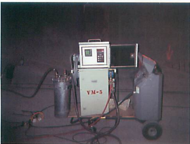
Fig. 4 – Measurement of Void Volume with Volumeter Capable of Compensating for Leaks
