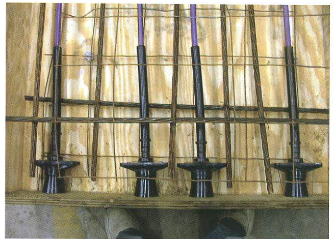
Fig. 2 - Close up of mock-up test set-up anchorages
