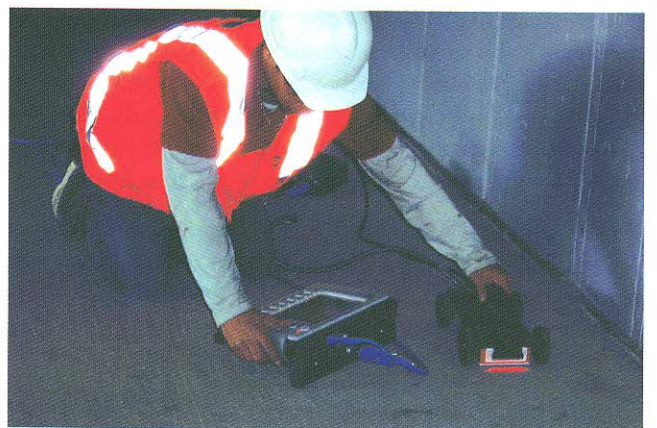
Fig. 3 - GPR scanning for tendon location
