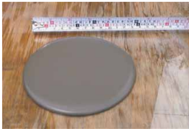
Fig. 13 - Slump Method Result for Grout 2
