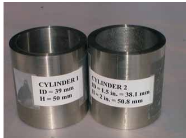
Fig. 11 - Cylinders for Slump Method
