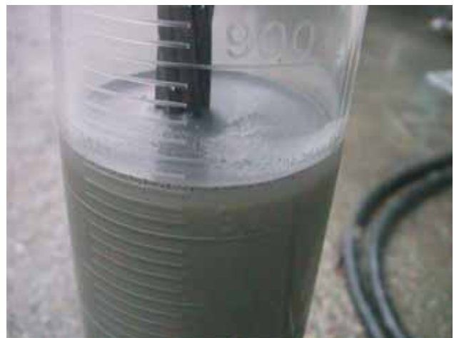
Fig. 17 - Bleeding (Discolor) of Grout 1 with Maximum Amount Water
