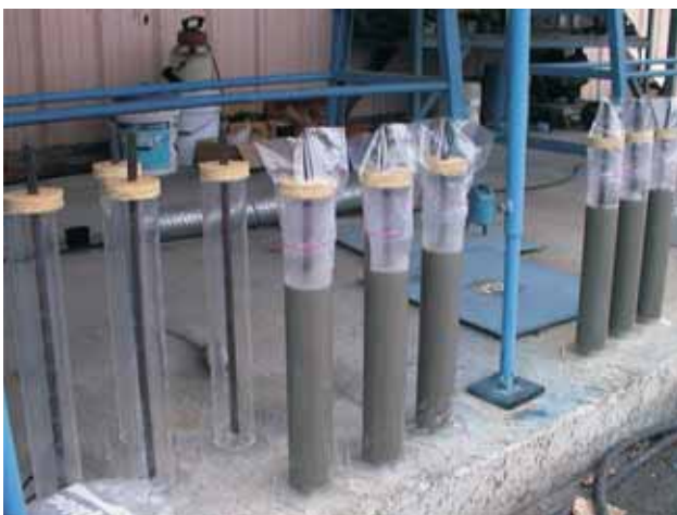
Fig. 16 - Test Set Up of Wick Induced Bleeding Test
