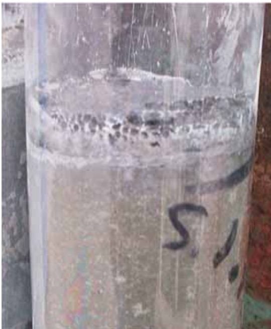
Fig. 21 - Close Up View of Segregation of Grout
