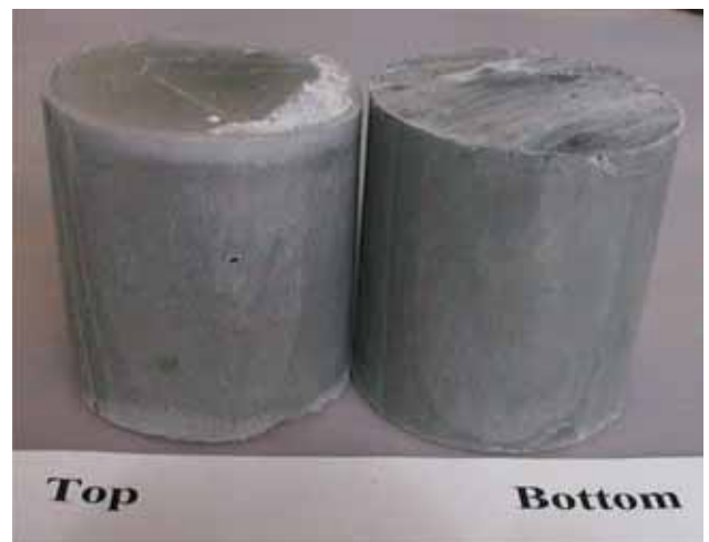
Fig. - 25 Non Segregation for Grout 2
