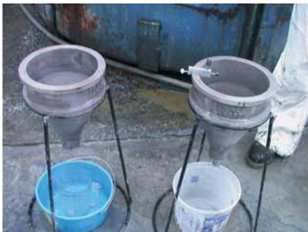
Fig. 8 - Modified Flow Cone on Left and Standard Flow Cone on Right Indicated with Grout Level
