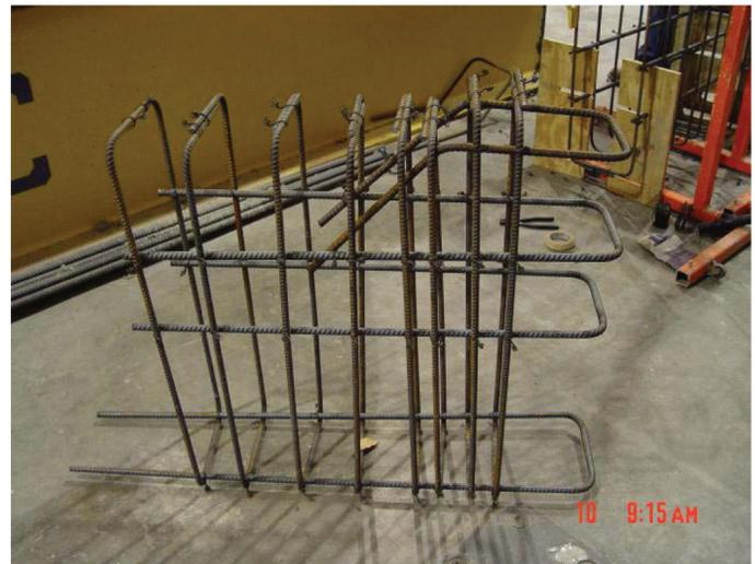
Fig. 5—End block reinforcement cage.
