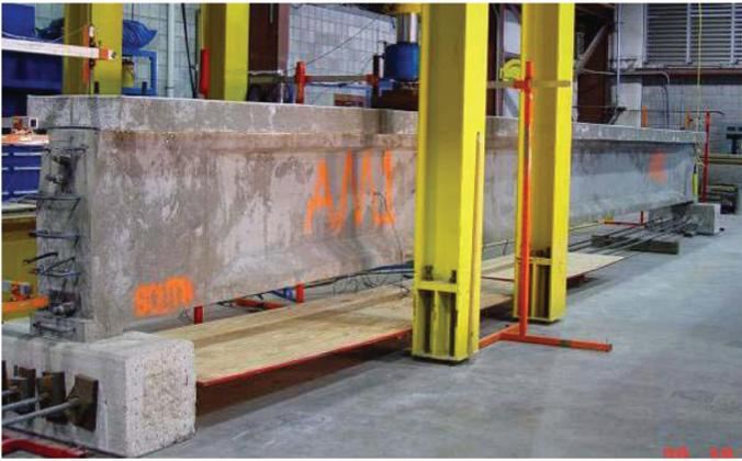
Fig. 7—Finished girder and deck.
