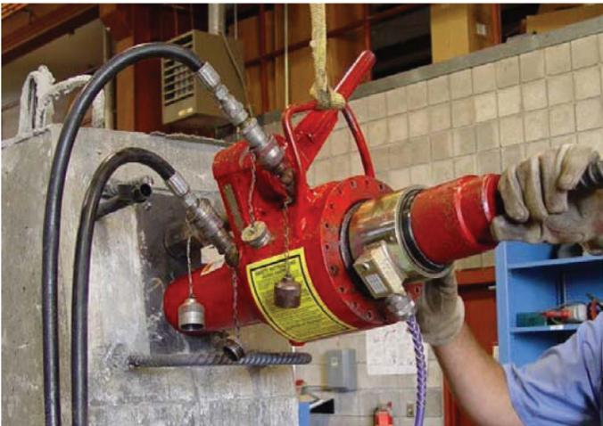
Fig. 8—Hydraulic jack used to stress PT bars.
