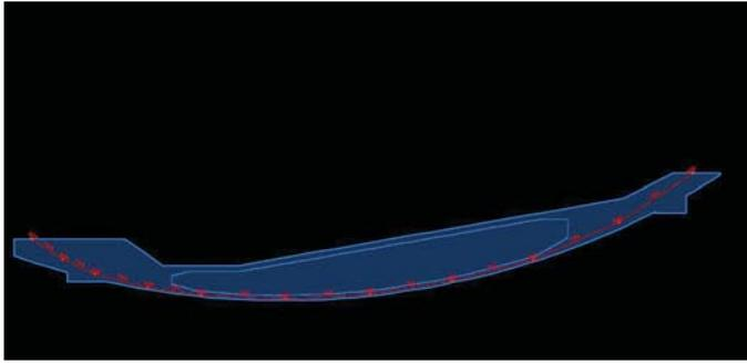
Fig. 3—Beam elevation with PT tendon in red.
