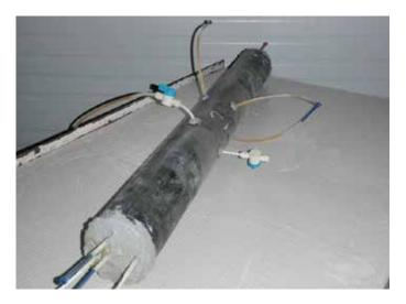
*Fig.* 7—*Impregnation being completed from midpoint of specimen.*
