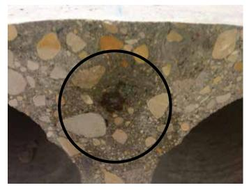
Fig. 4—Concrete surrounding a single seven-wire strand shows a radial pattern of impregnation.
