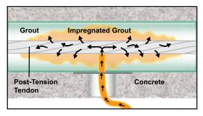
Fig. 2—Impregnation from a midpoint location on a tendon.
