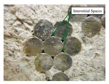
*Fig.* 3—*End view of a single strand from a tendon showing the inter-stitial spaces between the wires.*
