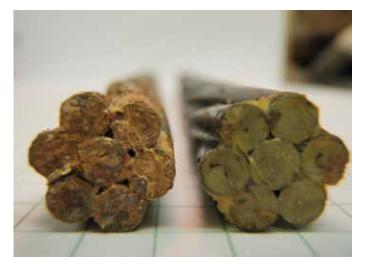
Fig. 18—Post-tensioned strand after exposure to salt-spray test. Left—untreated control; right—treated with impregnation material.
