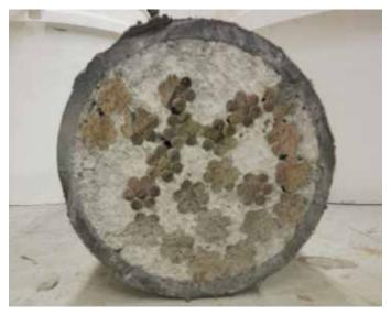
Fig. 5—End view of one FDOT tendon specimen, as received.
