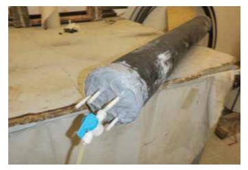
Fig. 6—Impregnation being completed from end of prepared specimen.
