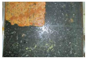
Fig. 17—Steel plate after exposure to salt-spray test Top left untreated control; top right and bottom—section treated with impregnation material.
