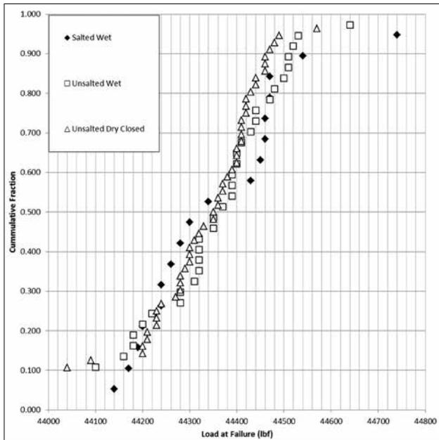
Fig. 5—Cumulative fraction of load at failure for all 216 strands comparison between salted and wetted strands, unsalted but wetted strands, and unsalted and dry strands.
