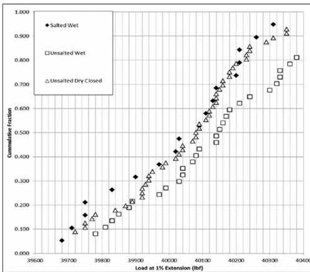
Fig. 6—Cumulative fraction of load at 1% extension for all 216 strands comparison between salted and wetted strands, unsalted but wetted strands, and unsalted and dry strands.
