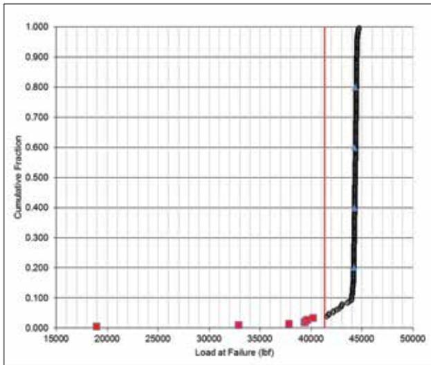
Fig. 2—Cumulative fraction of load at failure for all 216 strands. Red line indicates ASTM specification requirement. Red square symbols are indicative of invalid tests. Blue triangle symbols are for unexposed controls.
