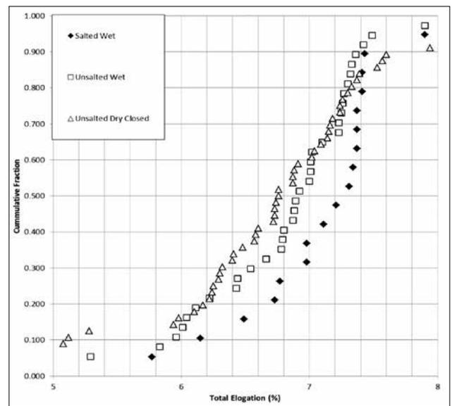
Fig. 7—Cumulative fraction of total elongation for all 216 strands comparison between salted and wetted strands, unsalted but wetted strands, and unsalted and dry strands.
