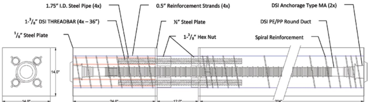
Fig. 1—Detensioning pile system design. PVC and flexible connection removed for clarity. (Note: 1 in. = 25.4 mm.)
