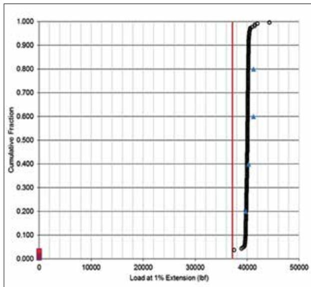
Fig. 3—Cumulative fraction of load at 1% extension for all 216 strands. Red line indicates ASTM specification requirement. Red square symbols are indicative of invalid tests. Blue triangle symbols are for unexposed controls.
