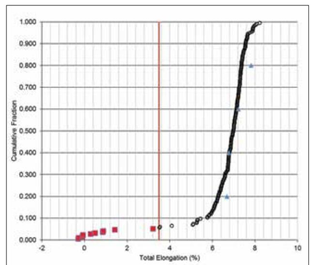
Fig. 4—Cumulative fraction of total elongation for all 216 Strands. Red line indicates specification requirement. Red square symbols are indicative of invalid tests. Blue triangle symbols are for unexposed controls.
