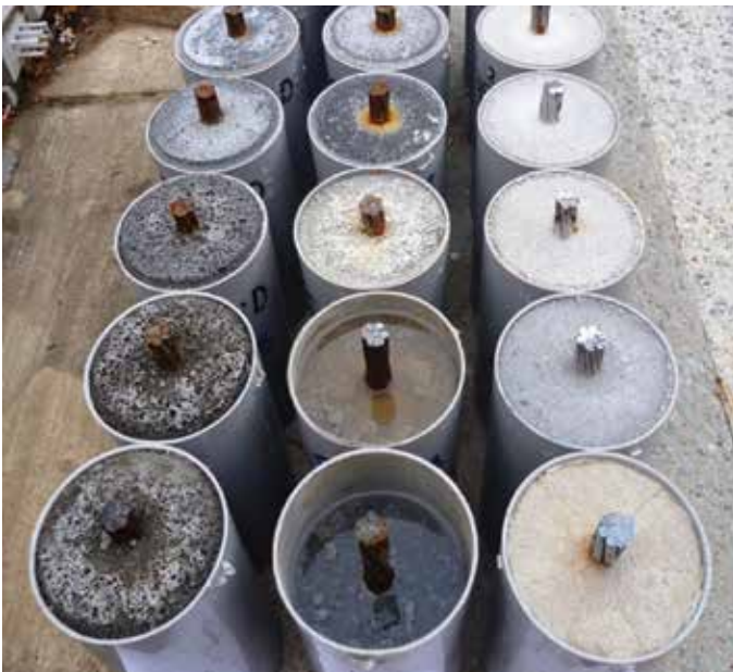
Fig. 14—Specimens cast with Grouts 1, 2, and 3 (right to left) and specified to 0.65 w/b (top to bottom).
