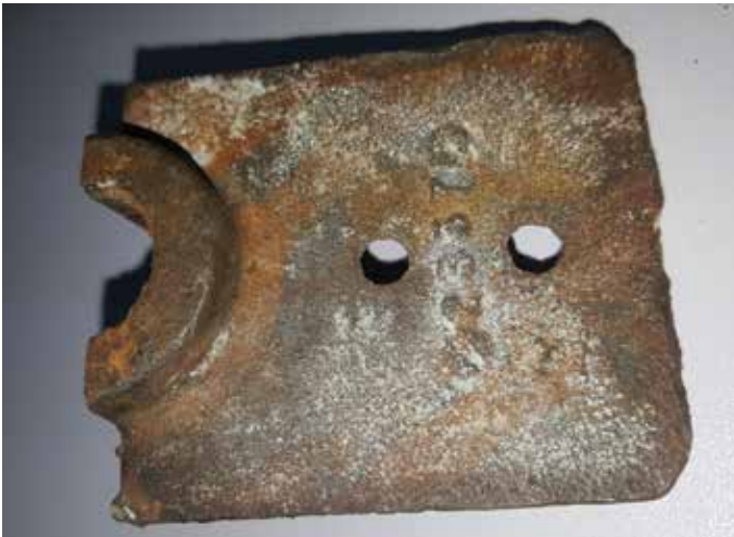
Fig. 3—Specimen No. 1: anchor, bearing side.
