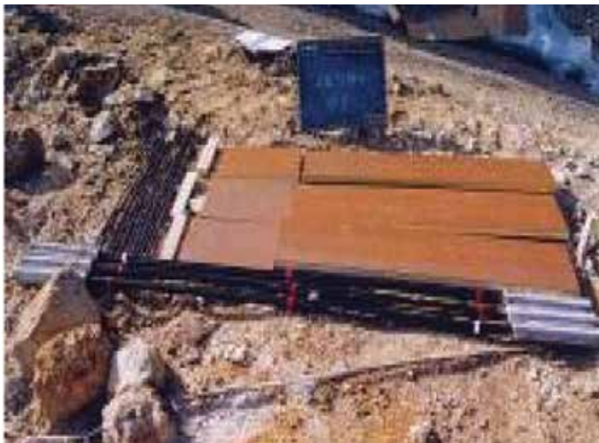
Exposure test and deterioration of sampled specimens at year 3
