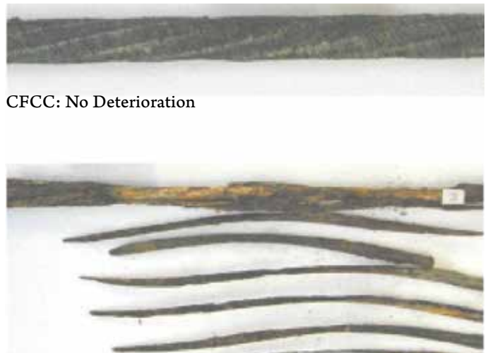
Steel strand: Crumbled by rust
