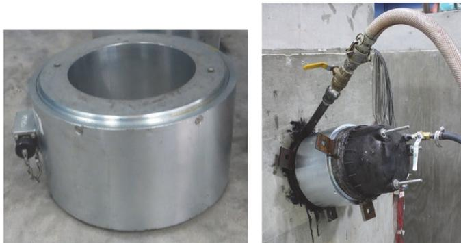
Fig. 2—Load cell (left) in line with anchorage during injection (right).
