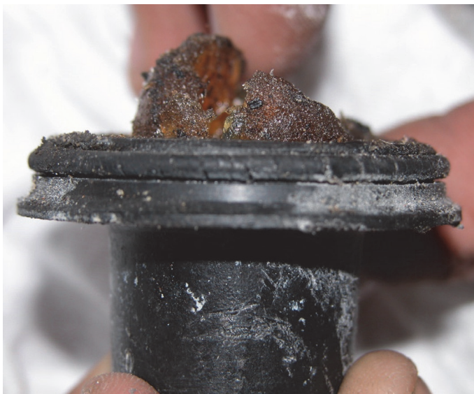
Fig. 3—Close-up of end cap O-ring with cracks.
