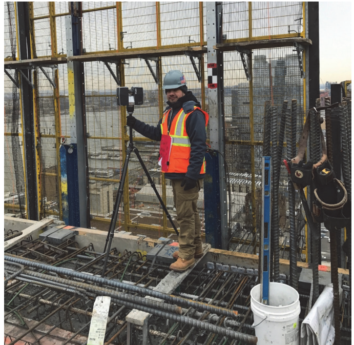
Fig. 7—FARO 3-D laser scanner used on project.
