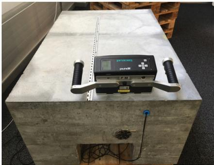
Fig. 5—Scanning with transducer perpendicular to the probe to create 3-D images.
