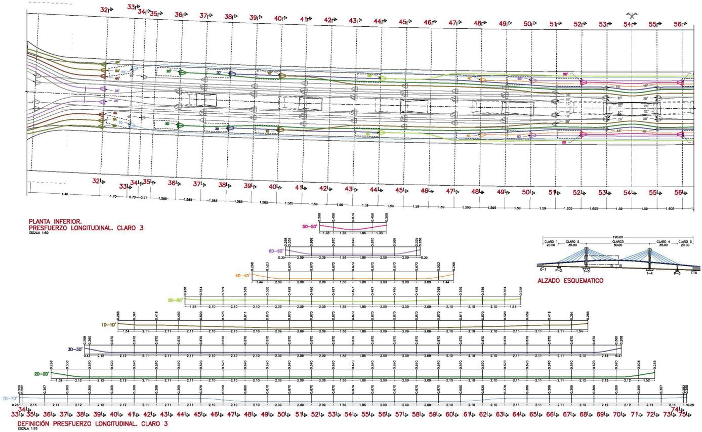
Fig. 6—Deck post-tensioning plan.
