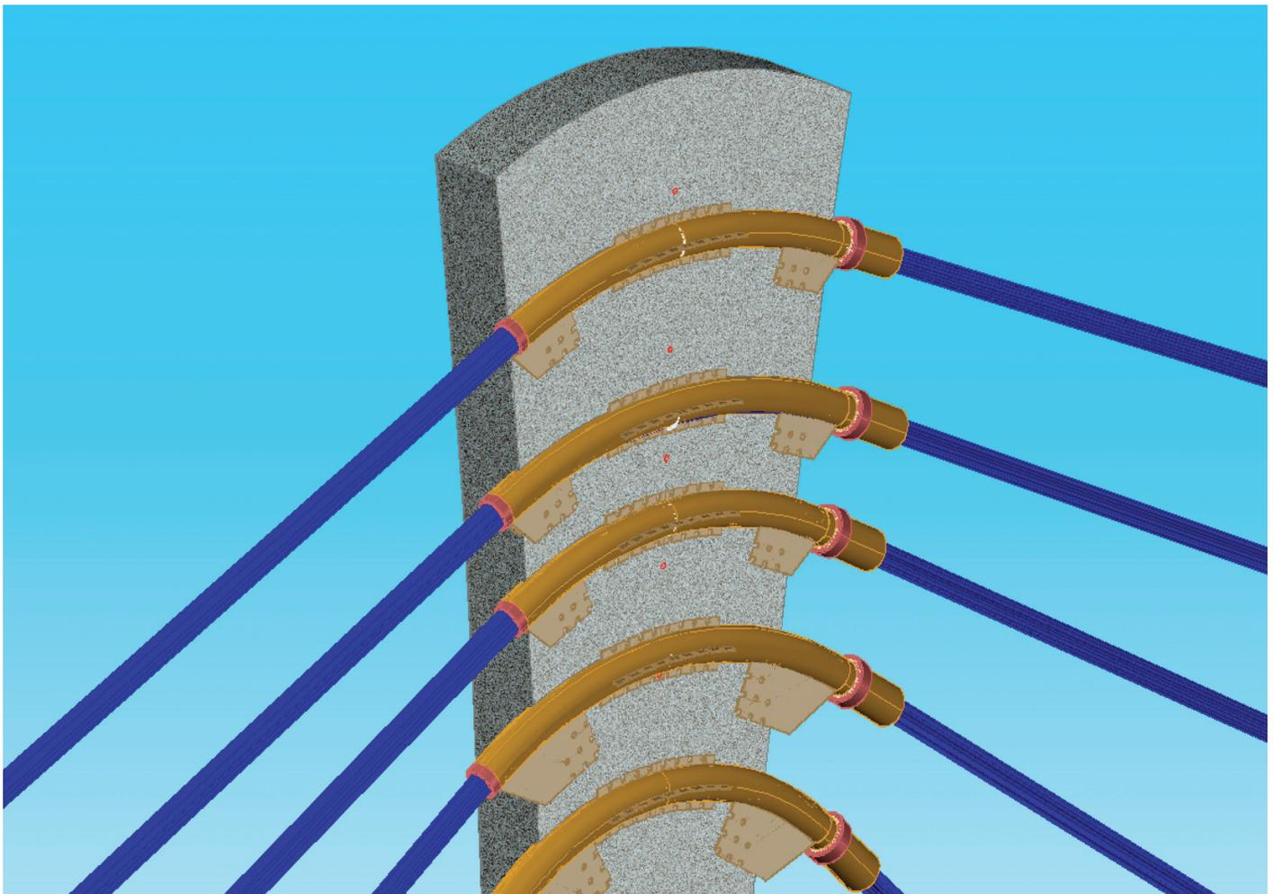
Fig. 3—Anchorage connection at pylon.
