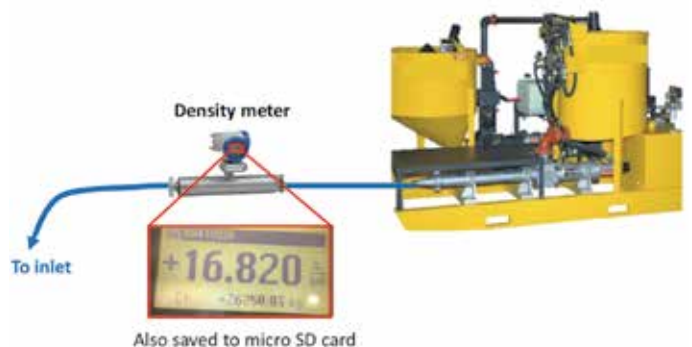
Fig. 1—Coriolis inline density meter setup.
