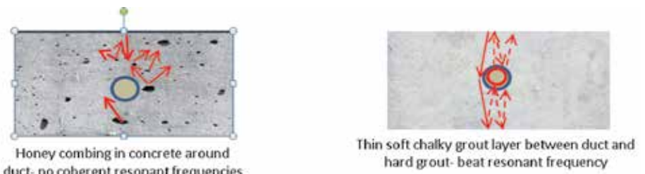
Fig. 6—Diffracted sonic wave paths.
