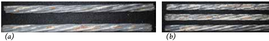
Fig. 12—Corroded strands near Port C of: (a) drying ISG specimen; and (b) drying TSG specimen.
