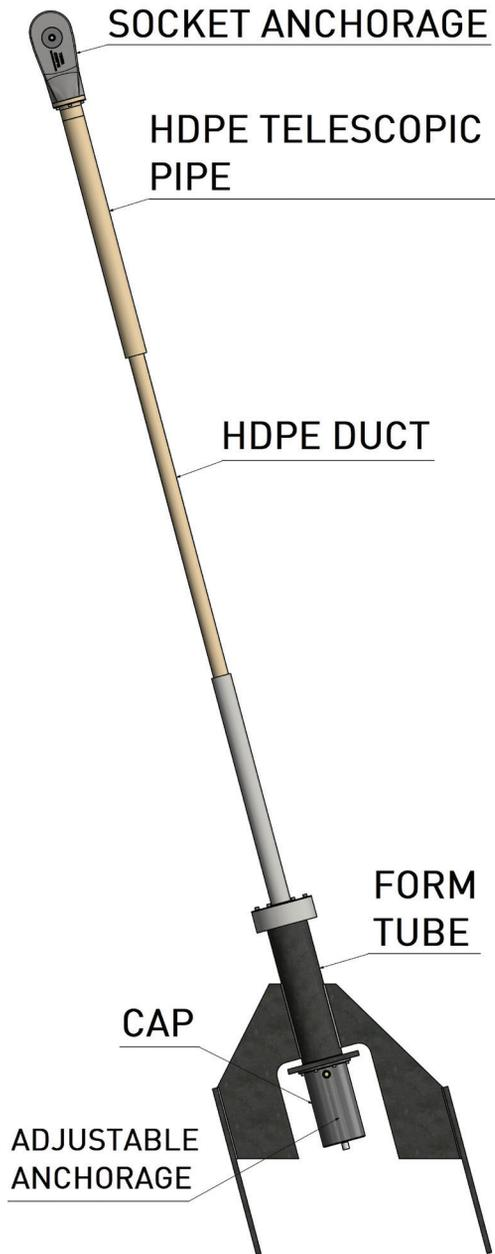
Fig. 1—Lateral view of stay cable system.
