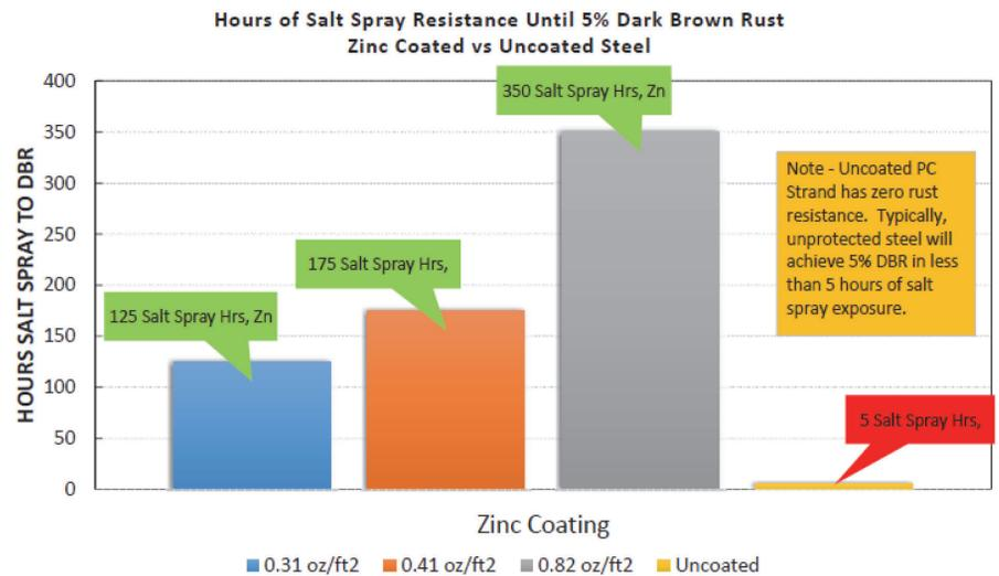
Fig. 3—Performance of galvanized strand in salt spray test. Note: 1 oz/ft<sup>2</sup> = 318 mL/m<sup>2</sup>.
