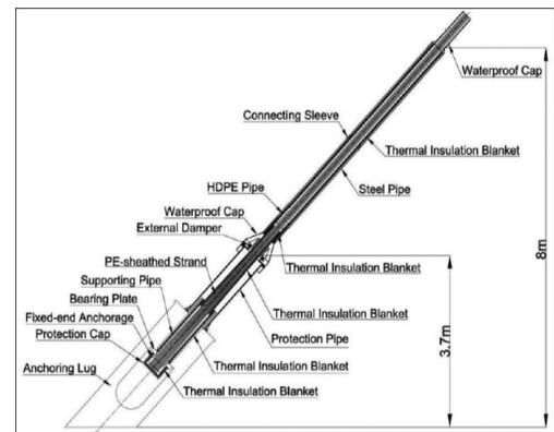
Fig. 5—Protection of stay cable at base.
