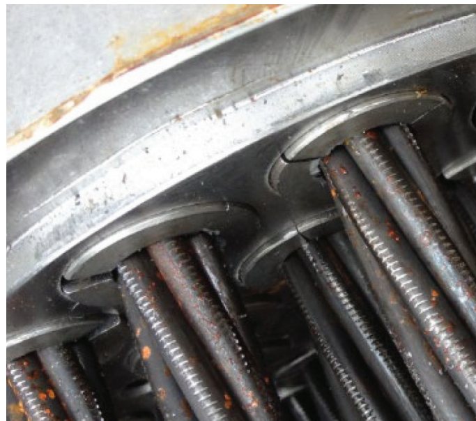
Fig. 3—Gripper indentations on multistrand system.
