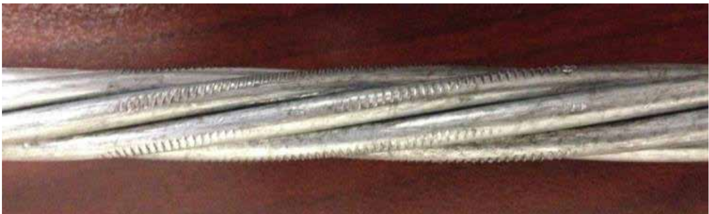
Fig. 2—Galvanized barrier cable with jack gripper marks after back stressing.
