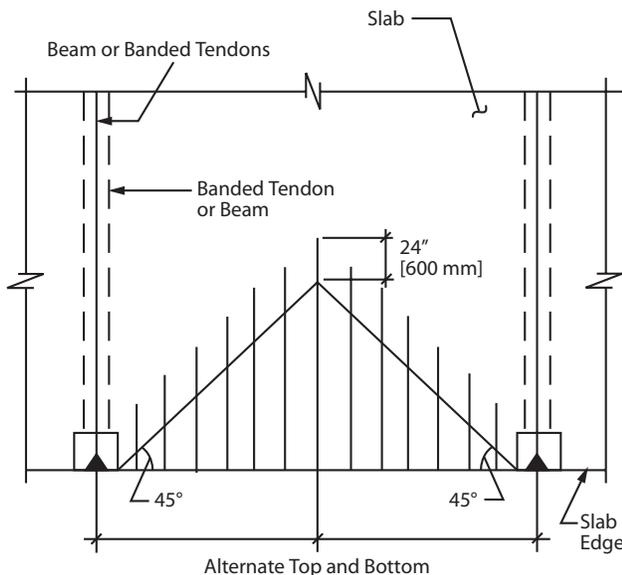
Fig. 3 – Arrangement of temperature and shrinkage reinforcement
