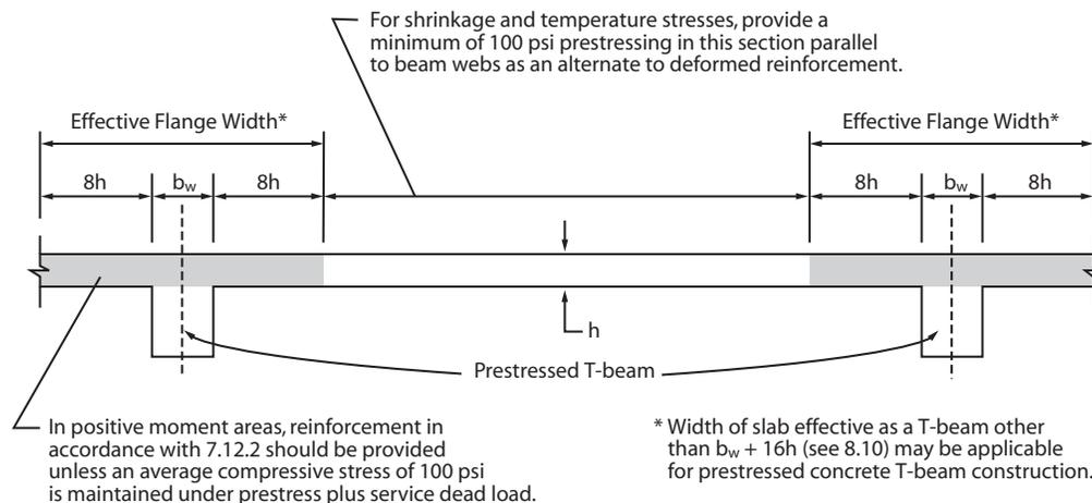
Fig. 1 – ACI Fig. R7.12.3—Prestressing used for shrinkage and temperature (Adapted from ACI 318-05)<sup>1</sup>
