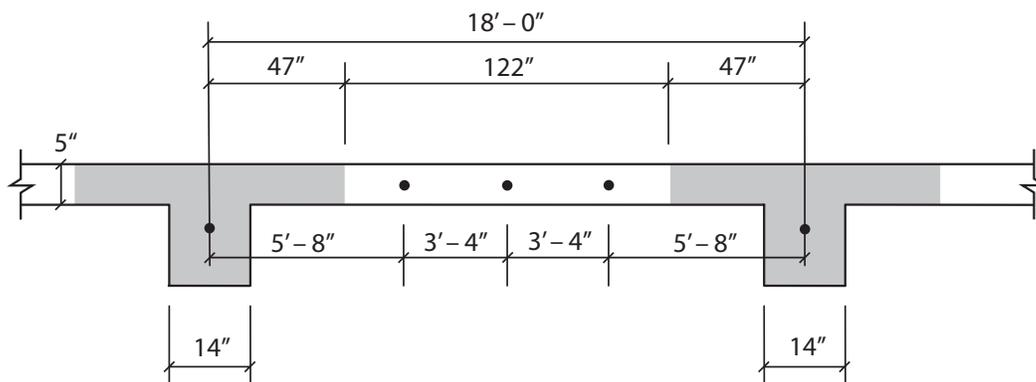
Fig. 2 – Example cast-in-place post-tensioned parking structure
