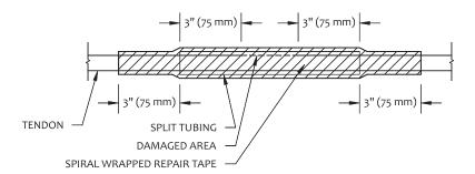
Note: Material used should be of suitable quality to allow for seal of aforementioned tubing method to be watertight
